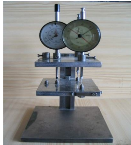
Fig.3 Fixing device wit so-called stop bar with timing gauge for measurement of dimensional changes
